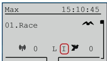
Please check the main screen if the cloud clocking function (I) is available on your device. The cloud clocking function requires that the latest firmware version of the BENZING Live Smart Hub as well as the BENZING M1 is installed.
