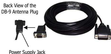
This cable, provided in a length of 10 m (30 ft), connects the PLB Antennas, the G2 Antennas and the BENZING Antenna Controller with EFA antennas to the BENZING M1. Moreover, the power supply unit is connected to this cable in order to supply the loft antennas and the BENZING M1 with power.
