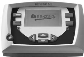
The BENZING M1 is the main device (the clock) of the complete system. All data that is entered or electronically registered is saved internally by the BENZING M1. When basketing a pigeon all data like ring number, secret number etc is saved in what is like a 'data safe'. This data remains stored until the race has been evaluated. During races or training sessions the arrival times of the pigeons in the loft are measured and saved in the BENZING M1.
