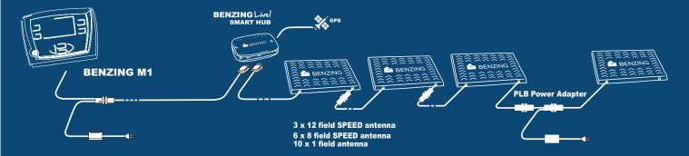
The system can be extended to a maximum of 64 SPEED or G2 antennas at any time using the PLB Power Adapter.
